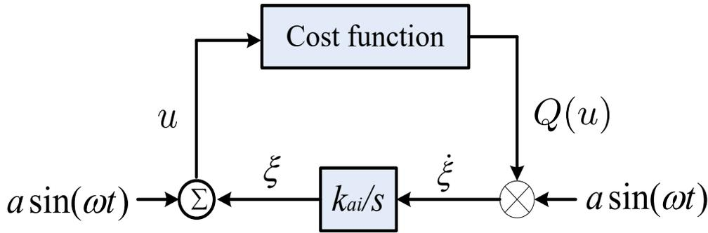
Block diagram of a static extremum seeking control algorithm
