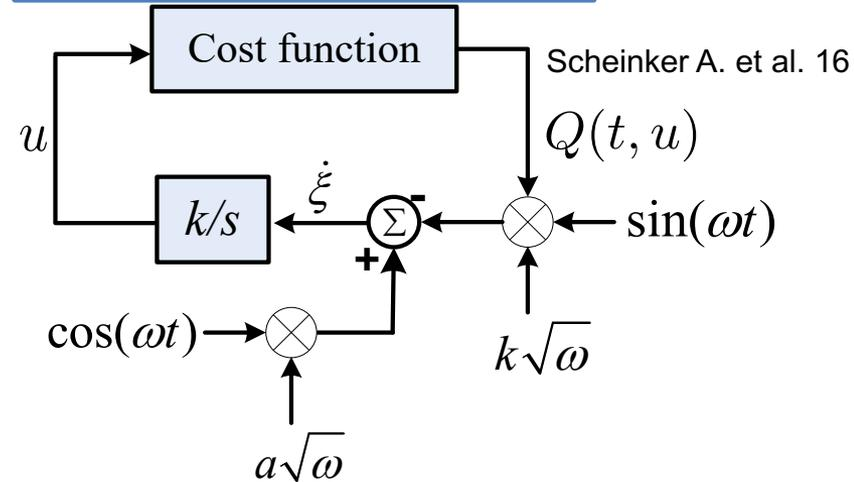
Block diagram of a functional extremum seeking control algorithm
