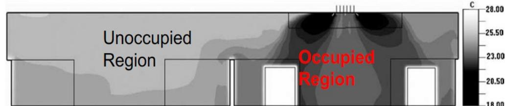
Hygiene applications: non-optimal vs optimal HVAC airflow to flush the virus out of the built environment
