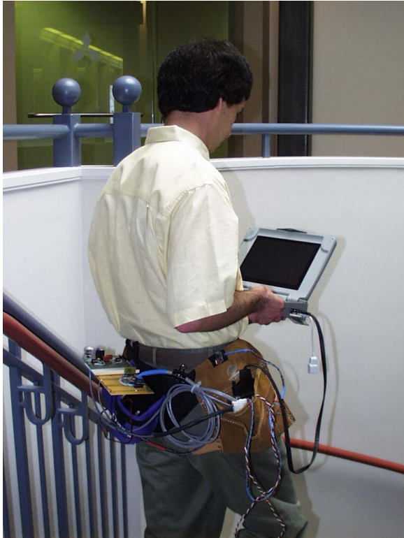
Figure 1: Initial prototype of wearable navigation system. User wears a “utility belt” which holds the sensor boards and a battery. The outputs of the sensors feed into a laptop on which the navigation program resides.
