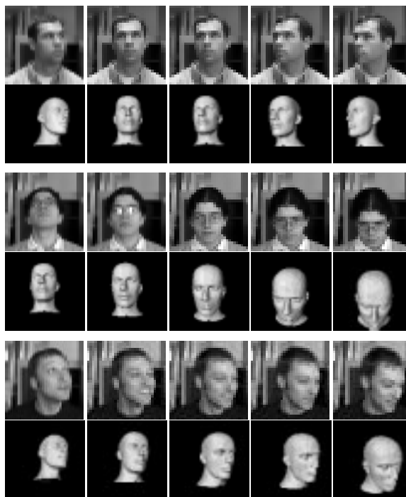
Figure 3: Segments of image sequences (not consecutive images) for different subjects, showing resilience to strong illumination gradients (top), specularities on spectacles (centre), and changing facial expression (bottom).
