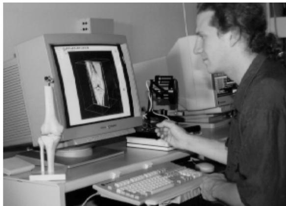
Figure 7. Prototype surgical simulation system. A 3D volumetric knee model has been generated from MRI images. A force feedback device allows the user to haptically explore the boney surfaces of the knee model while real-time polygon and volume-based rendering provide visual feedback to the user.
