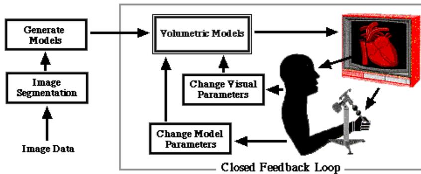
Figure 1: Surgical simulation system components. This system provides a closed feedback loop between the user and the simulator. The user can manipulate object models and observe the results both visually and haptically.
