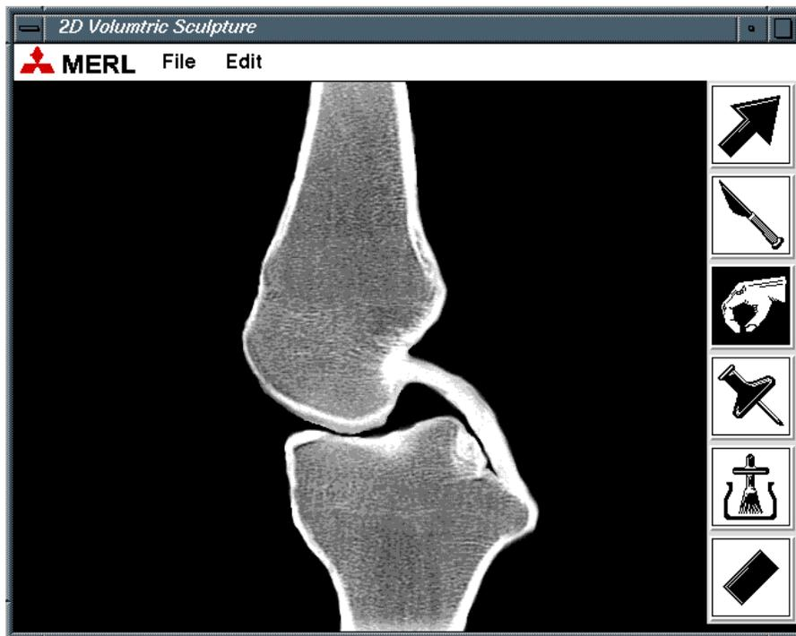
Figure 6. An interactive 2D application for manipulated 2D volumetric objects. Object elements can be moved (resulting in object translation), cut, grasped and moved (resulting in object deformation), tacked into place, glued together, and erased interactively using the computer mouse. Pointing and clicking on the buttons on the right side of the user interface switches between these modes.
