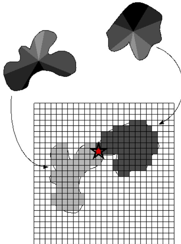
Figure 5. Simple collision detection for volumetric objects. Object elements are mapped into cells of the regular grid of the 3D occupancy map. As objects are moved, cells of the occupancy map are updated. If an element is written into a cell that is already occupied by a different object, a collision is detected.
