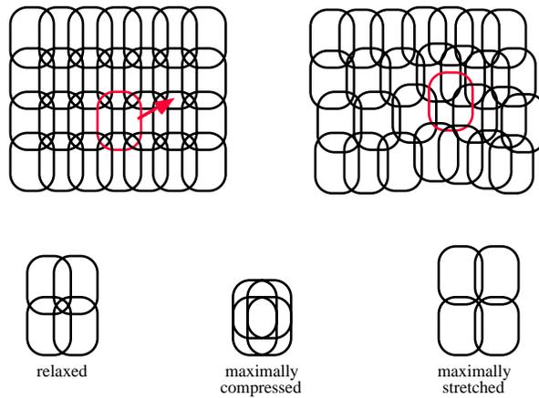
Figure 4. 2D ChainMail. a) and b) When one link of the 2D object is moved along the path of the arrow, its neighboring links move to satisfy maximum and minimum distance requirements between elements. Sets of 4 links at the bottom of the figure show relative link positions when the 4 links are in c) a relaxed state, d) a maximally compressed state, and e) a maximally stretched state.
