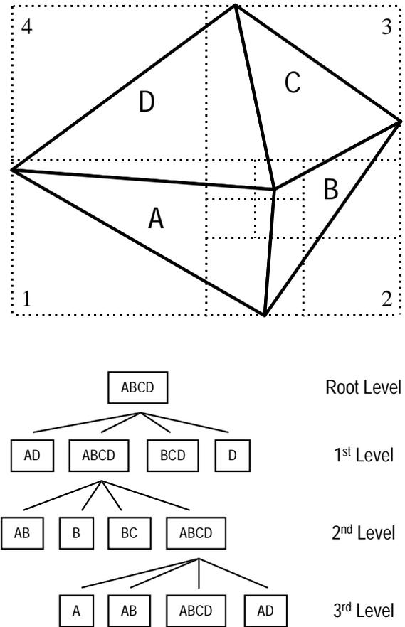
Figure 1. A simple terrain and QOTA quadtree.
