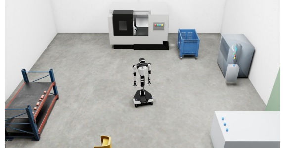
Fig. 5. The factory scene: the Galaxea R1, the three machines (M1–M3), the staging rack holding the work pieces, and the table of spare batteries. Panel close-ups are in Table. I.
