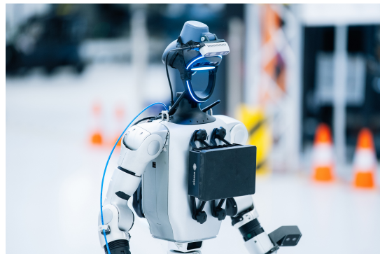
Fig. 6. Imaging radar prototype on a humanoid.
