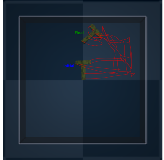
Fig. 2: The body is moved by an exploration policy to produce an identification image sequence and keypoints are tracked over the sequence by the TAPIR tracker.
