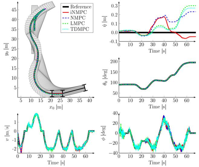
Fig. 4. One MC-simulation with the iNMPC (red), regular NMPC (blue), standard linear MPC (green) and TDMPC (cyan). *Top, left*: Configurations of the iNMPC response, and positional response  $(x_0(t), y_0(t))$  with all considered controllers. The wheelbases are drawn for the terminal configuration. *Top, right*: The lateral positional tracking error. *Center, right*: The trailer heading angle. *Bottom, left*: Velocity. *Bottom, right*: Steering angle.
