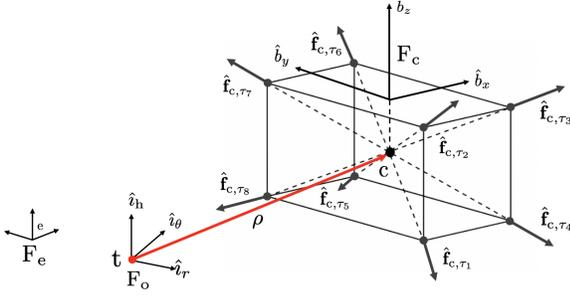
Figure 2: Chaser and thruster configuration schematics. The inertial, target orbital (Hill), and chaser frames,  $F_e, F_o, F_c$  are also shown.
