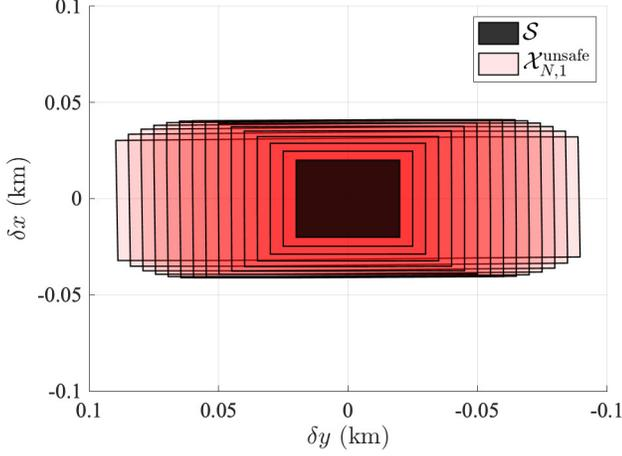
(a) Projections of the unsafe sets  $\mathcal{X}_{N,1}^{\text{unsafe}} \subset \mathbb{R}^6$  onto the  $\delta x$ - $\delta y$  plane for  $u_y = 0$ , i.e., the failure mode results in loss of along-track control. Because  $u_y = 0$  more states along  $\delta y$  are unsafe.
