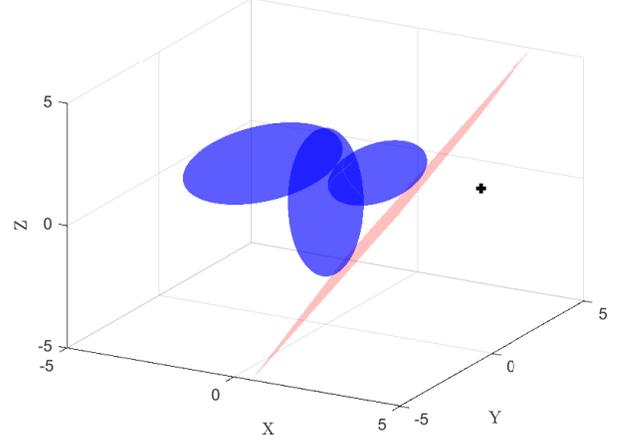
Figure 6: Example of Result 2 in  $\mathbb{R}^3$ . The blue ellipsoids represent sets to be avoided, while the red hyperplane separates the state marked by the black cross from the ellipsoids.
