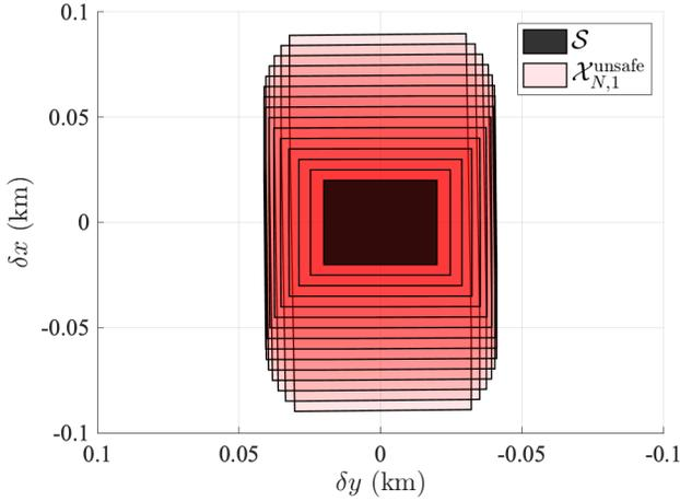
(b) Projections of the unsafe sets  $\mathcal{X}_{N,1}^{\text{unsafe}} \subset \mathbb{R}^6$  onto the  $\delta x$ - $\delta y$  plane for  $u_x = 0$ , i.e., the failure mode results in loss of radial control. Because  $u_x = 0$  more states along  $\delta x$  are unsafe.
