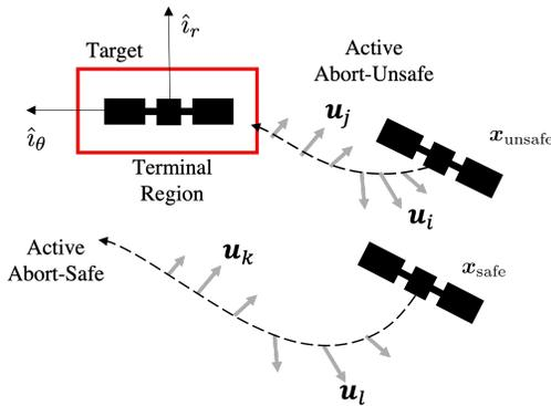
(b) For an active abort-unsafe state  $\mathbf{x}_{\text{unsafe}}$ , no control exists that keeps the chaser away of the terminal polytope, as opposed to an active abort-safe state  $\mathbf{x}_{\text{safe}}$
