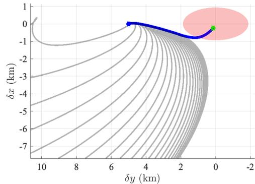
Figure 9: *Passively safe rendezvous* with respect to the AE, in red, from the along-track direction for a target in an eccentric orbit. States do not enter the AE within the safety horizon  $N$  under free-drift dynamics.
