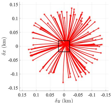
(b) Trajectories from multiple unsafe initial conditions  $\mathbf{x}_0 \in \mathcal{X}_{N,1}^{\text{unsafe}}(\mathcal{P}_f, \mathcal{U}_3)$ . The terminal region  $\mathcal{P}_f$  cannot be avoided.
