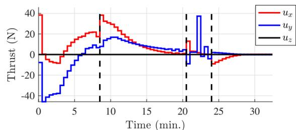
Figure 17: *Full rendezvous mission*, reaction of the control signal to the changing constraints due to the changing phases.
