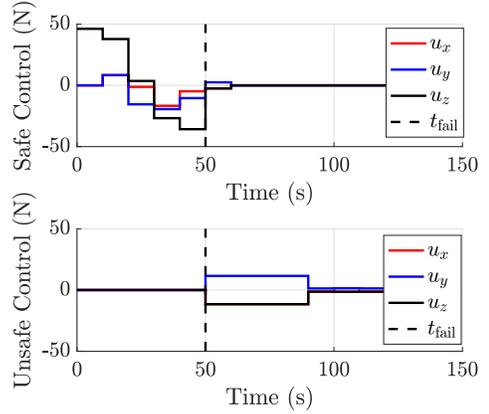
(b) Control histories for the safe and unsafe controllers. Vertical dash line shows  $t_{\text{fail}}$ .
