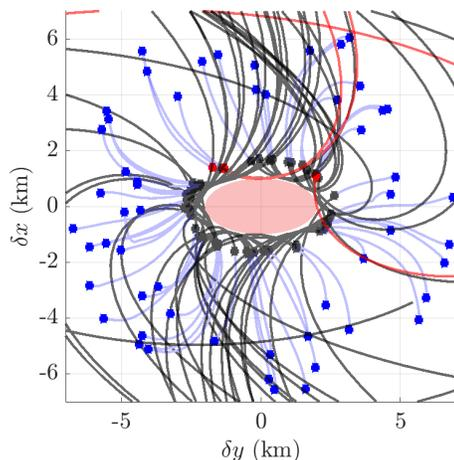
(a) Rendezvous from various initial conditions with nominal prediction model and nominal RS ( $\gamma = 1$ ). Passively safe approaches (blue), free-drift trajectories (black), failure events (black marker); 3/55 trajectories (red) entered (briefly) the AE.
