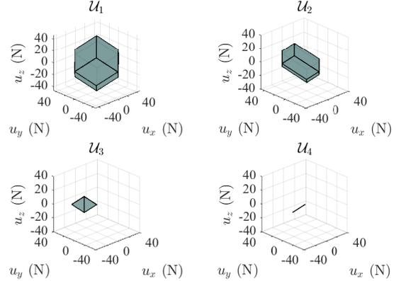
Figure 3: Admissible control sets for different thrust modes. Top left:  $\mathcal{M}_i = \mathcal{I}$ , all thrusters functional. Top right:  $\mathcal{M}_i = \{1, 2, 3\}$ , thrusters 1, 2, 3 working. Bottom left:  $\mathcal{M}_i = \{7, 8\}$ . Bottom right:  $\mathcal{M}_i = \{8\}$ .
