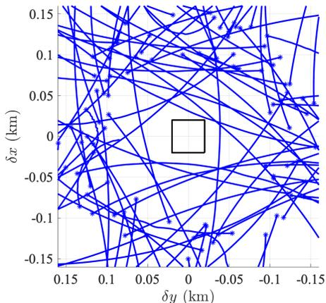
(a) Trajectories from safe initial conditions,  $\mathbf{x}_0 \in \mathcal{X}_{N,1}^{\text{safe}}(\mathcal{P}_f, \mathcal{U}_3)$ . The terminal region  $\mathcal{P}_f$  is avoided.
