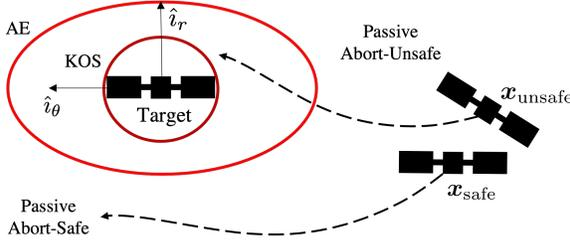
(a) For a passive abort-unsafe state  $\mathbf{x}_{\text{unsafe}}$ , the natural dynamics takes the chaser into the AE and KOS, as opposed to a passive abort-safe state  $\mathbf{x}_{\text{safe}}$ .
