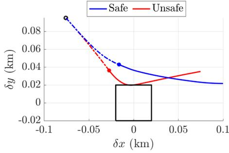
(a) Rendezvous towards the terminal region (black) for safe (blue) and unsafe (red) controllers. The black circle and marks show the initial and failure states, respectively. Dashed and solid lines are states before and after propulsion failure, respectively.
