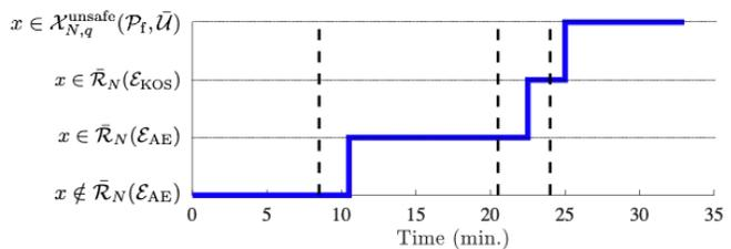
Figure 16: *Full rendezvous mission*. The trajectory enters the unsafe set of each phase only after the next phase has started.
