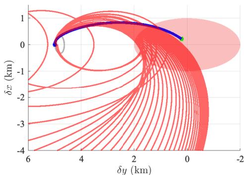
Figure 8: *Passively unsafe rendezvous* with respect to the AE from the along-track direction for a target in an eccentric orbit. States along the trajectory enter the AE under free-drift dynamics.
