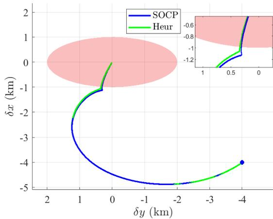
Figure 7: Comparing the rendezvous resulting from SOCP and radial projection ellipsoid-based passive safety constraints.
