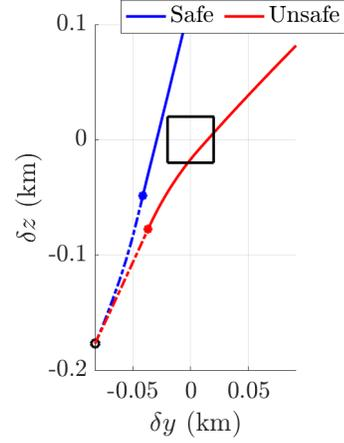
(a) Rendezvous to the terminal set (black) for the safe (blue) and unsafe (red) controllers. The black circle and marks are the initial and failure states, respectively. Dashed and solid lines are states before and after propulsion failure, respectively.
