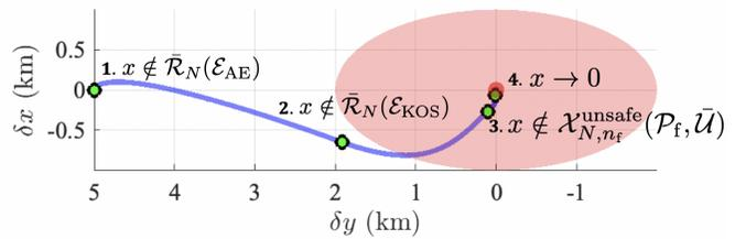
Figure 15: *Full rendezvous mission*, safe trajectory with annotated phases and corresponding safety specifications. Each phase begins at a green circle.
