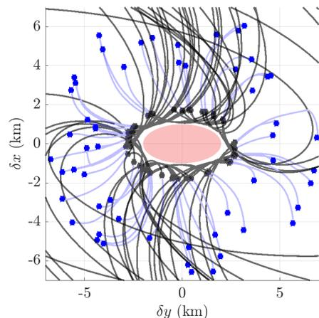
(b) Rendezvous from various initial conditions with nominal prediction model and inflated RS ( $\gamma = 1.1$ ). Passively safe approaches (blue), free-drift trajectories (black), failure events (black marker). No trajectory (even briefly) enters the AE.
