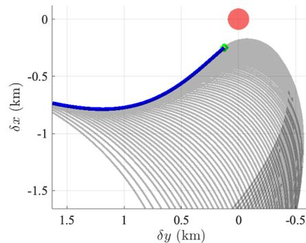
Figure 10: *Passively safe rendezvous* with respect to the KOS, in red, from the along-track direction for a target in an eccentric orbit. States do not enter the KOS within the safety horizon  $N$  under free-drift dynamics.
