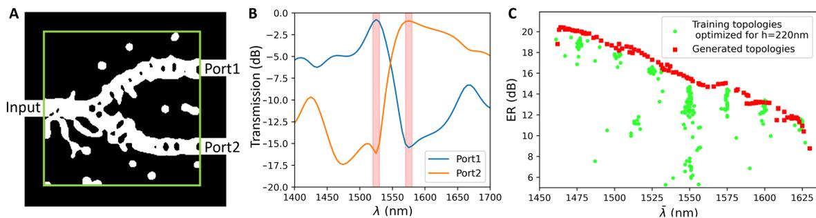
Fig. 1. (A) Optimized device topology (black: silicon oxide background, white: silicon waveguide, box: optimization area of  $4.5 \times 4.5 \mu\text{m}^2$ ) and (B) transmission spectra of an example device generated by DNN. (C) Performance of densely generated topologies (red squares) from DNN trained with a sparse set of topologies optimized for 220 nm-thick devices (green dots).
