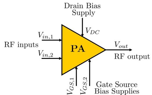
Fig. 1. Block diagram of dual-input Doherty PA.
