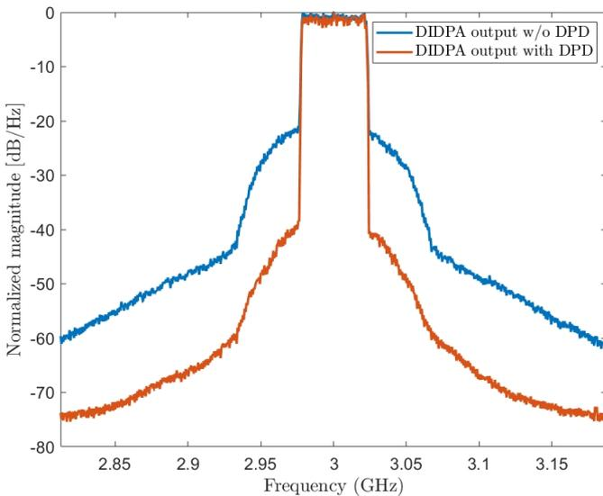
Fig. 5. Spectra of the output signal of DUT without and with DPD.
