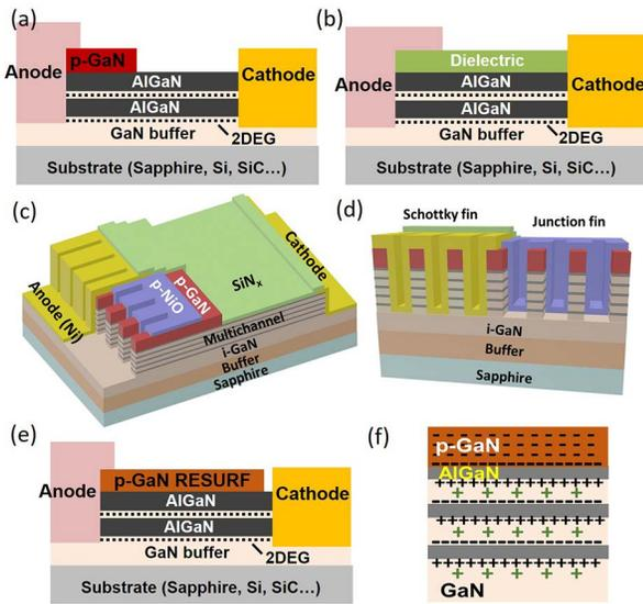
FIG. 6: Schematic of multi-channel diodes with (a) p-GaN termination and (b) field-plate termination. 3-D (c) side-view schematic and (d) cross-sectional view of a multi-channel AlGaIn/GaN SBD with the junction-fin-anode. Schematic of (e) the RESURF multi-channel diode, and (f) the charge balance in the structure.
