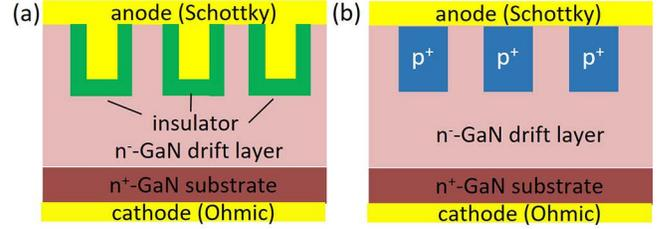
FIG. 3: Schematic of vertical GaN (a) TMBS and (b) JBS rectifiers.
