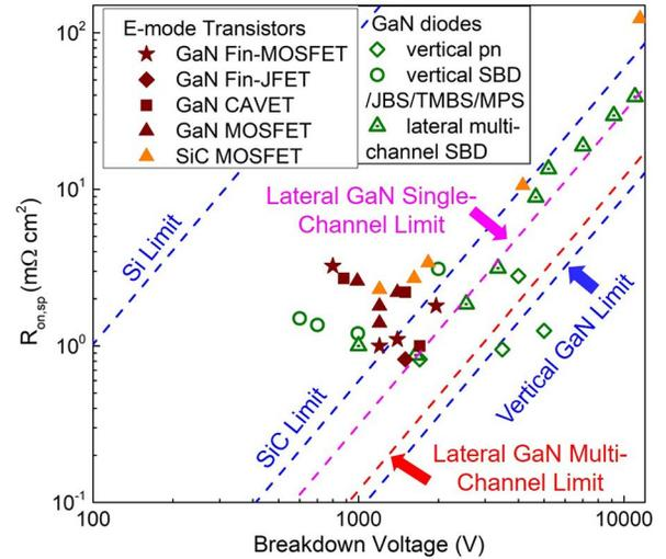
FIG. 7: Specific  $R_{\text{ON}}$  v.s. BV performance of the state-of-the-art MV/HV vertical and lateral GaN diodes and transistors. The performance limits of 1-D unipolar Si devices, SiC devices, lateral single-channel and multi-channel GaN devices, and vertical GaN devices are also included.
