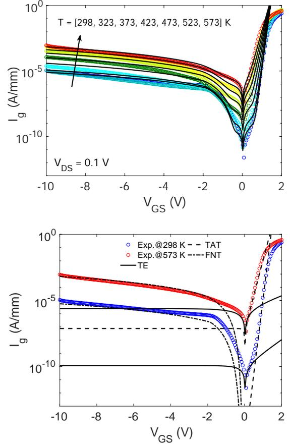
FIG. 24: (up) Gate leakage versus gate bias at different temperatures. Symbols indicate experimental data while solid lines correspond to model fits. The drain bias is fixed at 0.1 V. Reproduced with permission from the International Conference on Simulation of Semiconductor Processes and Devices (SISPAD), 2020. Copyright 2020 IEEE. (bottom) Contribution to gate leakage at 573 K and 298 K arising from trap assisted tunneling (TAT), Fowler Nordheim tunneling (FNT), and thermionic emission (TE).
