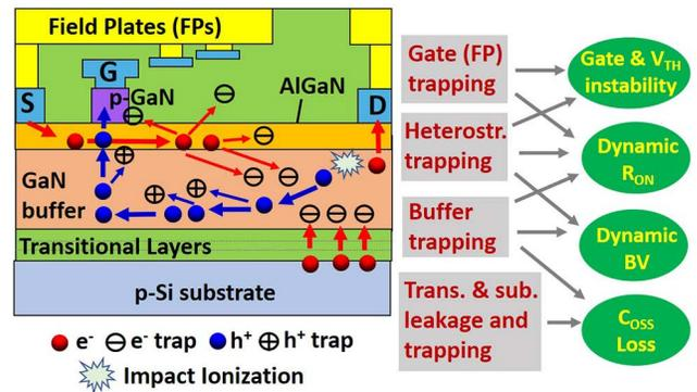
FIG. 10: Schematic of the electron/hole dynamics and trapping inside a p-gate HEMT during high-voltage power switching, with the illustration of different trapping mechanisms and their correlation with several device phenomena.
