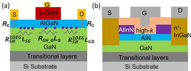
FIG. 8: (a) Illustration of the  $R_{ON}$  components and channel electron concentrations in a ULV p-gate HEMT. (b) Schematic of Intel's ULV MOS-HEMT with a partial barrier recess (i.e., AlInN recess under the gate).
