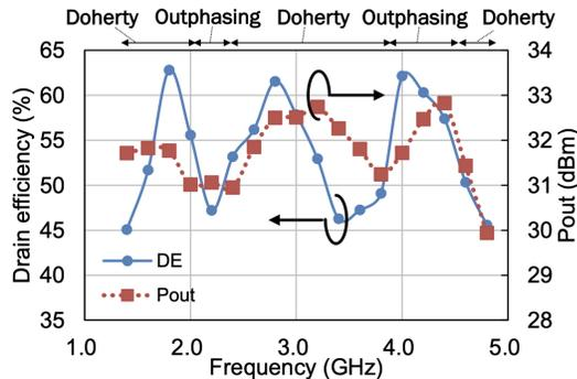
FIG. 17: (a) Machine learning assisted dual-input mixed-mode GaN PA. (b) its measured performance over ultra-wide bandwidth.<sup>138,139</sup> Reproduced with permission from IEEE/MTT-S International Microwave Symposium Proceeding. Copyright 2019 IEEE.
