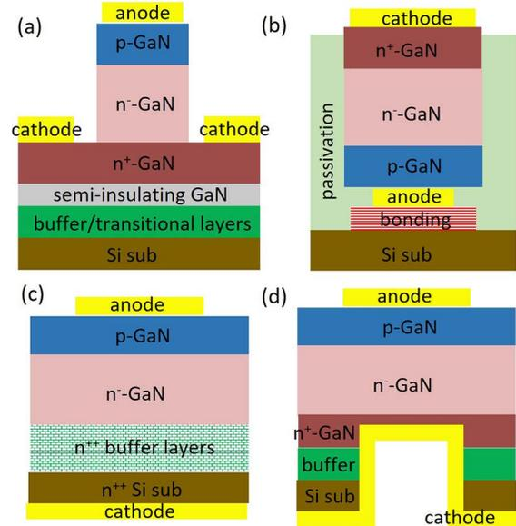
FIG. 5: Schematic of (a) quasi-vertical GaN-on-Si diodes and the fully-vertical diodes through (b) layer transfer, (c) buffer doping, and (d) selective removal of substrate and buffer layers.
