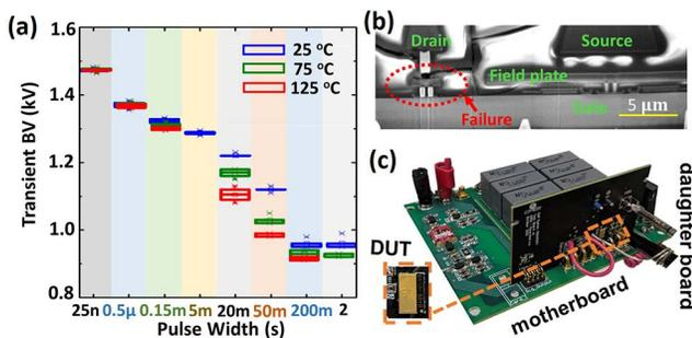
FIG. 11: (a) Box plots of the dynamic BV of SP-HEMTs failed at different pulse widths and temperatures. (b) Cross-sectional SEM image of the device failed in 25 ns pulse, showing the failure location at the drain side. (c) Photo of the test setup with a motherboard/daughter-board configuration. Reproduced with permission from IEEE International Electron Devices Meeting 23.3 (2020) and IEEE Electron Device Lett. 42, 505 (2021). Copyright 2020 and 2021 IEEE.
