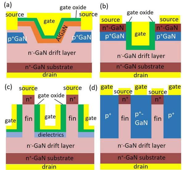
FIG. 4: Schematic of vertical GaN (a) CAVET, (b) trench MOSFET, (c) Fin-MOSFET, and (d) Fin-JFET.
