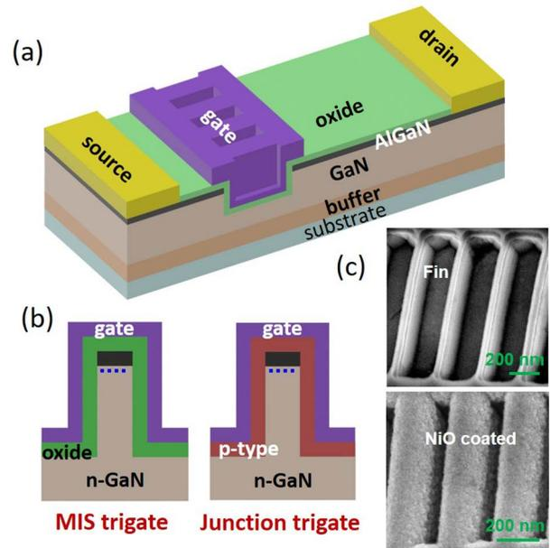
FIG. 9: (a) 3-D schematic of a tri-gate GaN HEMTs and (b) cross-sectional schematic of a MIS-type tri-gate and a junction-type tri-gate. (c) Scanning electron microscopy (SEM) images of the NiO-wrapped AlGaIn/GaN fins in a junction tri-gate.
