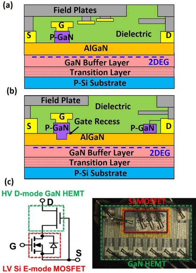
FIG. 2: Schematic or decapped photos of four mainstream commercial GaN HEMTs: (a) SP-HEMT, (b) GIT, and (c) cascode GaN HEMT.
