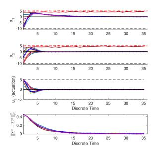
Fig. 4. PAC-MPC simulations with state-dependent measurement quality. Closed-loop state and input trajectories for different initial system states and fixed initial environment uncertainty. Environment state  $x^e$  (dash, red), constraints due to environment mean and covariance, i.e.,  $-\gamma(\mathcal{M}^e)$ , (solid, dark red), setpoint  $r^x$ ,  $r^u$  (solid, black), deterministic constraints (dash, black).
