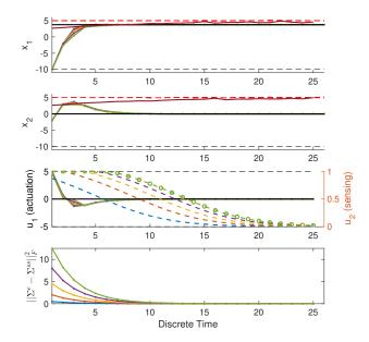
Fig. 3. PAC-MPC simulations with input-dependent measurement quality. Closed-loop state, input, and covariance trajectories for different initial environment uncertainties and fixed initial system state. Environment state  $x^e$  (dash, red), constraints due to environment mean and covariance, i.e.,  $-\gamma(\mathcal{M}^e)$ , (solid, dark red), setpoint  $r^x$ ,  $r^u$  (solid, black), deterministic constraints (dash, black), perception input (dash, orange axis).
