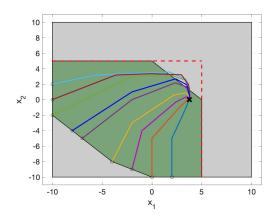
Fig. 2. PAC-MPC simulations with input-dependent measurement quality. Phase plot of closed-loop state trajectories for different initial system states and fixed initial environment uncertainty. Constraints due to the actual environment state  $x^e$  (dash, red), initial region of recursive feasibility (green), setpoint (cross, black).
