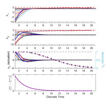
Fig. 1. PAC-MPC simulations with input-dependent measurement quality. Closed-loop state, input, and environment covariance trajectories for different initial system states and fixed initial environment uncertainty. Environment state  $x^e$  (dash, red), constraints due to environment mean and covariance, i.e.,  $-\gamma(\mathcal{M}^e)$ , (solid, dark red), setpoint  $r^x$ ,  $r^u$  (solid, black), deterministic constraints (dash, black), perception input (dash, cyan axis).
