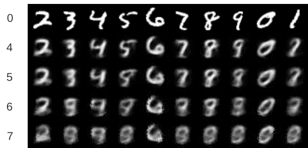
Fig. 5. UAE attack images for several values of \ell_2 distance, \epsilon . For large \epsilon , the UAE attack is stronger and can potentially confuse a human eye.
