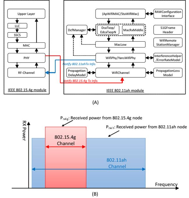
Figure 5: Sub-1 GHz Band Coexistence Simulator Model Interface
