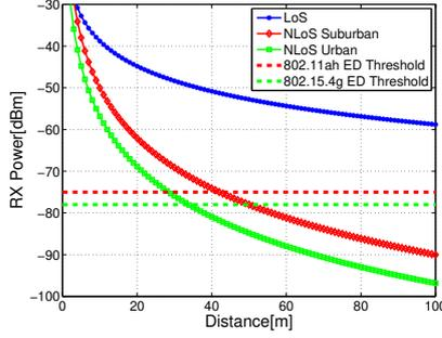
Figure 6: ITU-R P.1411-9 Propagation Model
