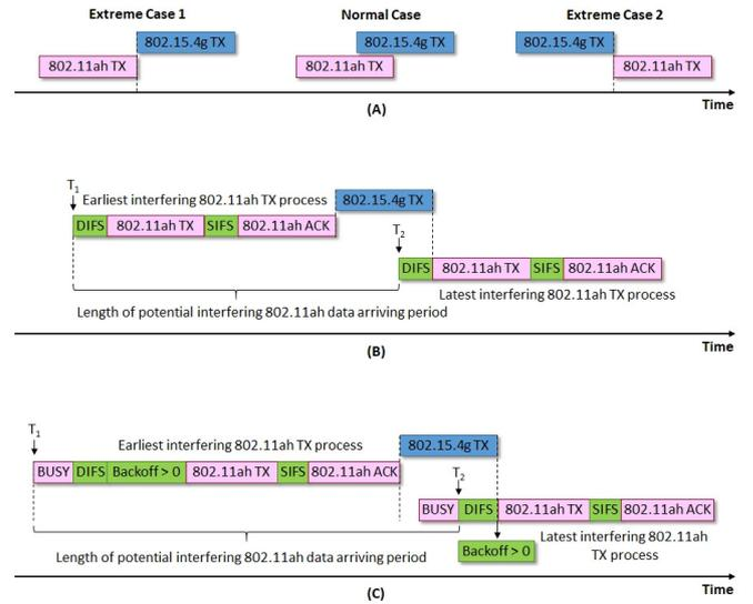
Figure 4: 802.11ah TX interfering with 802.15.4g TX
