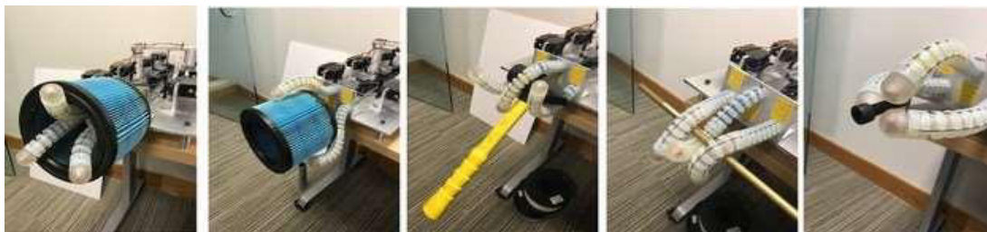
Illustration 1: various gripping modes available with a 3D SLA printed multi-tentacular (Cthulhu-morphic) gripper with each tentacle having two independently actuated 2-DoF sections (4 DoF per tentacle, 12 DoF total).
