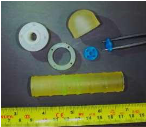
Illustration 4: Samples of each part type for the final version 5 design – a fairlead and a 25mm OD guide ring (translucent white, Formlabs Durable), a friction cap and an 80mm x 19mm OD / 13mm ID core tube (fluorescent yellow, Formlabs Elastic) and two spacer / cable guide 12.3mm x 5mm ellipsoids (blue, Formlabs Tough). All prints made at 0.1mm resolution.
