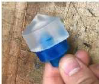
Illustration 6: Fine Grasp (0.0 mm radius) fingertip mounted on a fairlead, printed in Formlabs Elastic material.
