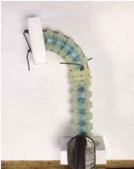
Illustration 3: Testing range of motion with a desktop jig on a two-section tentacle of design version 5.
