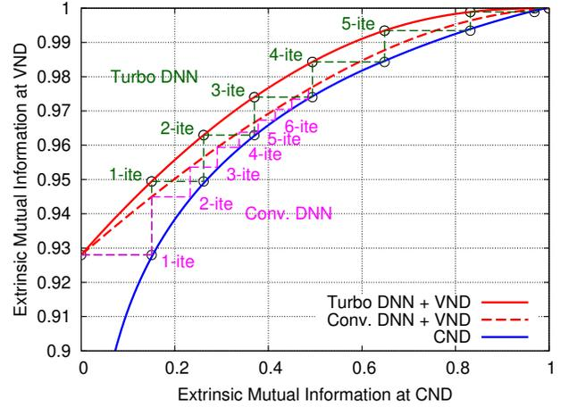
Fig. 11. Combined EXIT chart [52] of DNN-TEQ & LDPC decoder for DVB-S2 code rate  $9/10$  (DP-16QAM in 16-span DM links at  $-2$  dBm).
