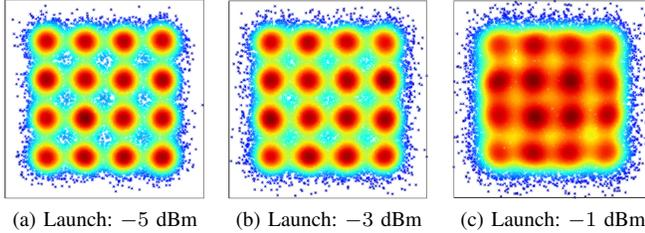
Fig. 4. Residual distortion of DP-16QAM after LE at 16-span NZDSF links.
