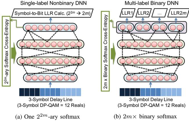
Fig. 5. Nonbinary and binary DNN equalizers for DP- $2^m$ QAM.
