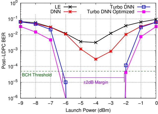
Fig. 13. BER performance for DP-64QAM 8-span NZDSF DM links (LDPC code rate 5/6, 8-iteration BP decoding).
