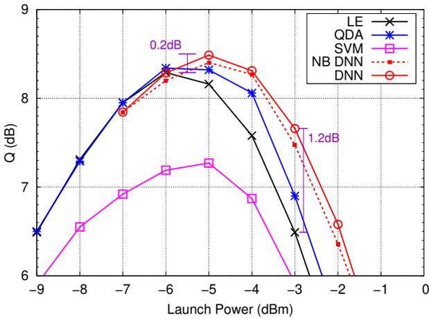
Fig. 6. Q factor comparisons for DP-4QAM 50-span NZDSF.
