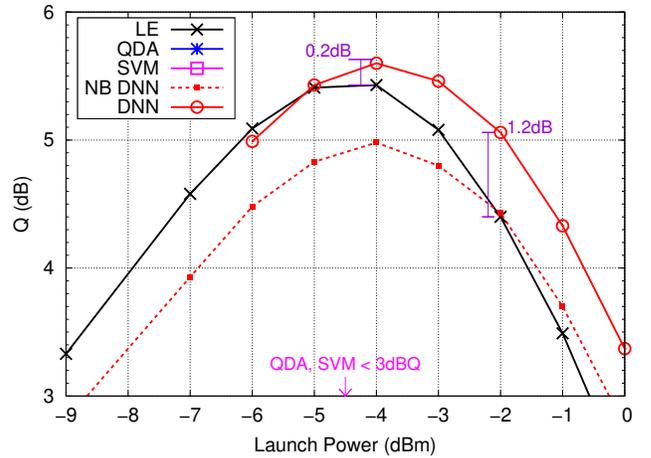
Fig. 8. Q factor comparisons for DP-64QAM 8-span NZDSF.
