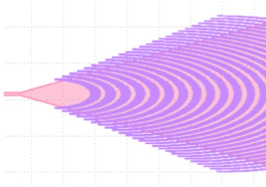
Figure 5. Mask pattern for the InP grating coupler, where purple patterns indicate the etched grating region, and orange patterns indicate the ridge region where the InP cladding layer is not etched away. The total ridge taper length is 200  $\mu\text{m}$ .
