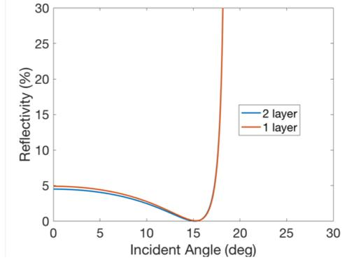
Figure 3. Reflectivity at the facet with a single layer  $\text{Si}_3\text{N}_4$  or two layer  $\text{Si}_3\text{N}_4/\text{SiO}_2$  coating optimized for  $15^\circ$  as a function of the angle of incidence.
