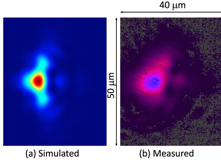
Figure 7. (a) Simulated and (b) measured beam pattern projected on a plane  $40 \mu\text{m}$  below the InP grating plane. The grating chirp parameters are  $\Delta_x = -1.6 \times 10^2 / \mu\text{m}$ , and  $\Delta_y = -1.2 \times 10^2 / \mu\text{m}$ .
