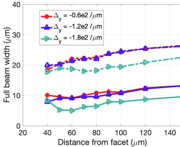
Figure 8. (Full beam width in the y direction (13.5% and 50% of the peak power) as a function of distance from facet.  $\Delta_y$  is the grating chirp parameter in the y direction.
