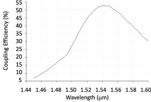
Figure 4. Coupling efficiency from the InP waveguide into the silicon waveguide through a pair of InP and Si grating couplers calculated from a 2D FDTD simulation.
