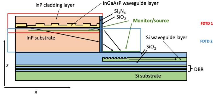
Figure 1. Schematic of the proposed grating coupler based integration scheme. The whole region was used for 2D FDTD simulations. When two-step 3D FDTD simulations were performed, the electric field obtained in the first FDTD step (FDTD1) is used for the source of the second step (FDTD2).
