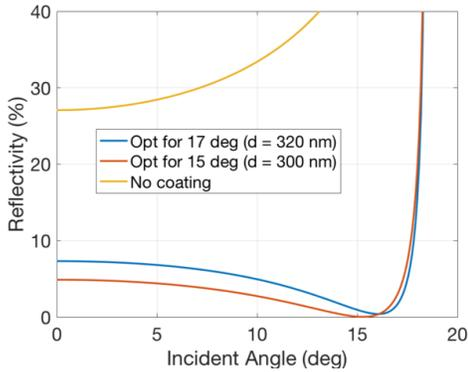
Figure 2. Reflectivity at the facet with a single layer  $\text{Si}_3\text{N}_4$  film optimized for  $15^\circ$  and  $17^\circ$  as a function of the angle of incidence.
