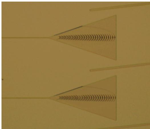
Figure 6. Top view microscope image of the fabricated InP grating coupler.
