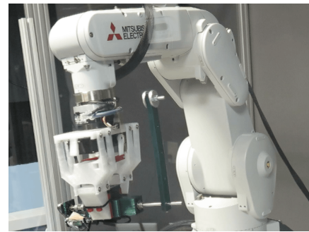
Fig. 5: The Furuta Pendulum (3D printed in color green) held in the wrist joint of the robot at the swing-up position reached using the learned controller.
