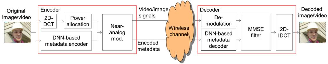
Fig. 1. Overview of the proposed soft delivery, employing DNN-based metadata encoder/decoder.
