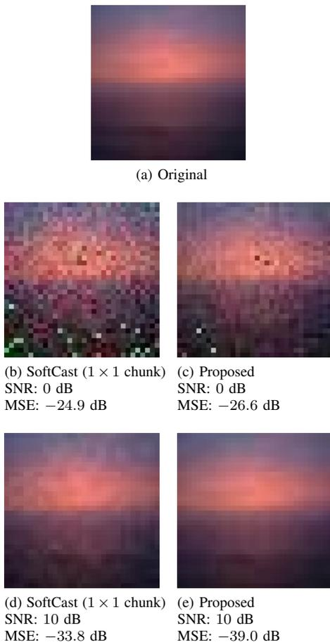
Fig. 4. Snapshot of a reconstructed image from CIFAR-100 at SNRs of 0 dB and 10 dB.
