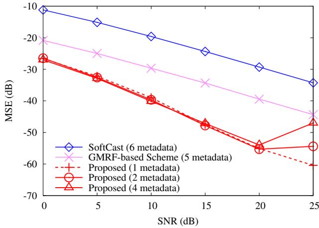
Fig. 6. MSE performance of the proposed and existing soft delivery schemes with different amount of metadata  $m$  as a function of wireless channel SNR.
