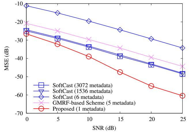
Fig. 3. MSE performance of the proposed and existing soft delivery schemes as a function of wireless channel SNR.
