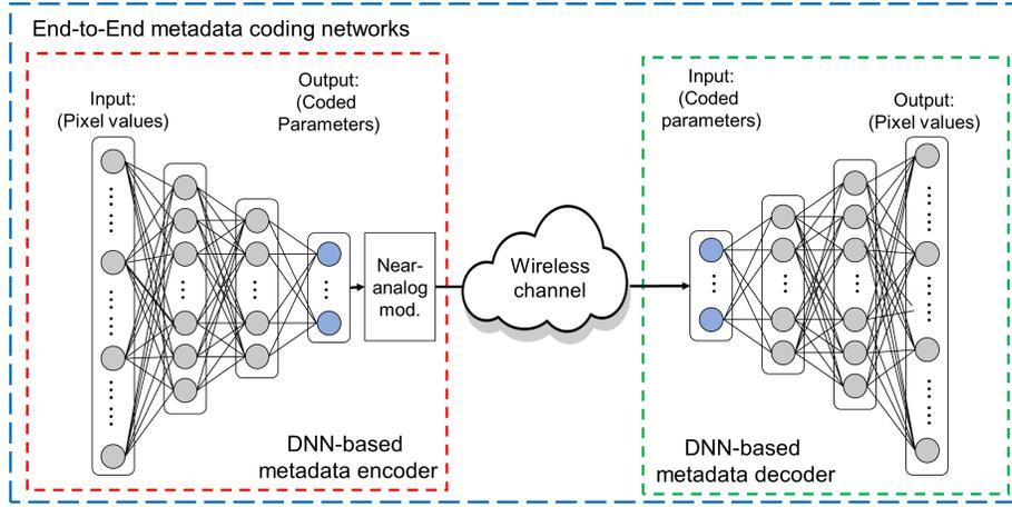
Fig. 2. End-to-End DNN-based metadata coding/decoding networks, analogous to denoising auto-encoders [17].
