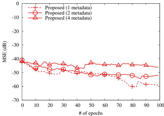
Fig. 7. Learning curves of the proposed schemes with different amount of metadata  $m$  as a number of epochs at wireless channel SNR of 25 dB.
