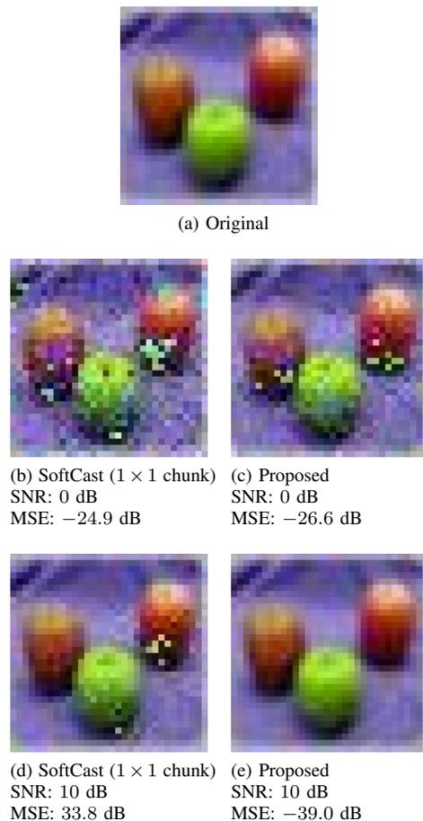
Fig. 5. Another snapshot of the reconstructed image from CIFAR-100 at SNRs of 0 dB and 10 dB.
