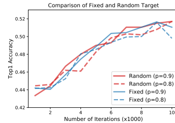
Figure 9: Comparison of the proposed RIDE algorithm using fixed target image (blue curves) or target image with random Gaussian noise (red curves). We show the comparison with random loss masking ratio of p = 0.9 and p = 0.8 .
