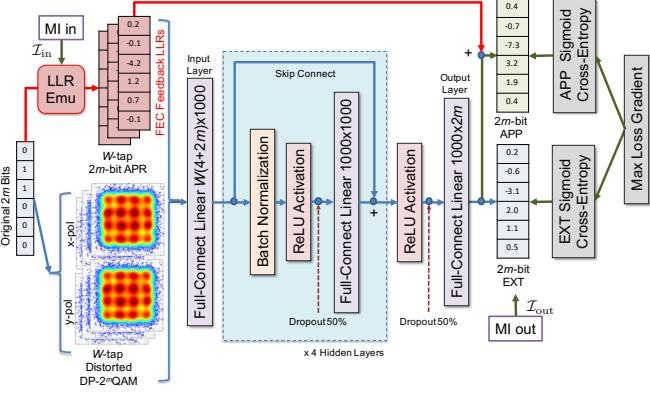
Fig. 3: DNN-TEQ architecture and min-max-loss training.
