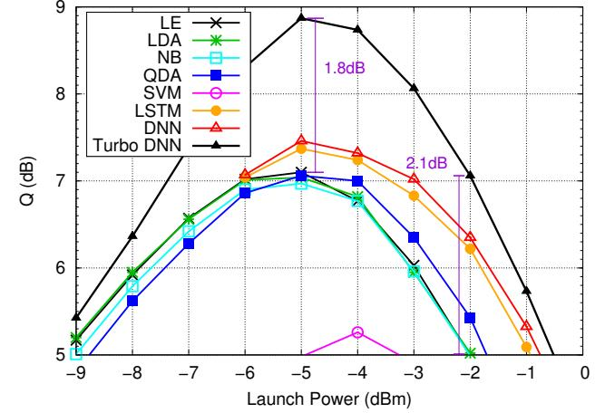
Fig. 7: Single-iteration DNN-TEQ for DP-16QAM 16-span NZDSF (DVB-S2 LDPC code of rate 8/9).
