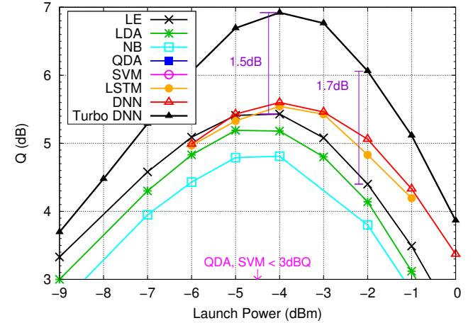
Fig. 8: Single-iteration DNN-TEQ for DP-64QAM 8-span NZDSF (DVB-S2 LDPC code of rate 4/5).
