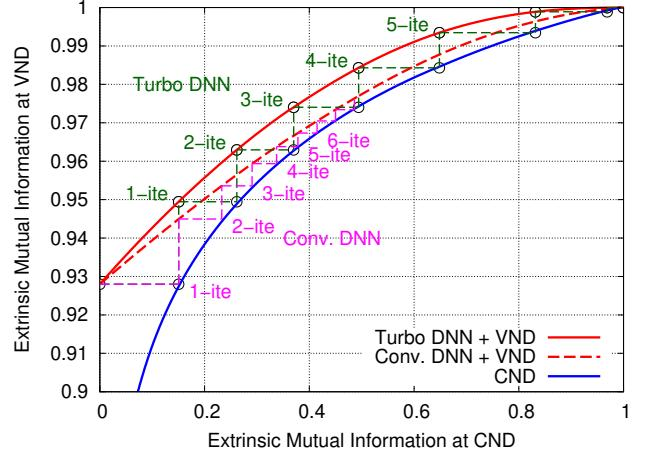
Fig. 5: Combined EXIT chart [26] of DNN-TEQ & LDPC decoder for DVB-S2 code rate 9/10 (DP-16QAM in 16-span DM links at  $-2$  dBm).
