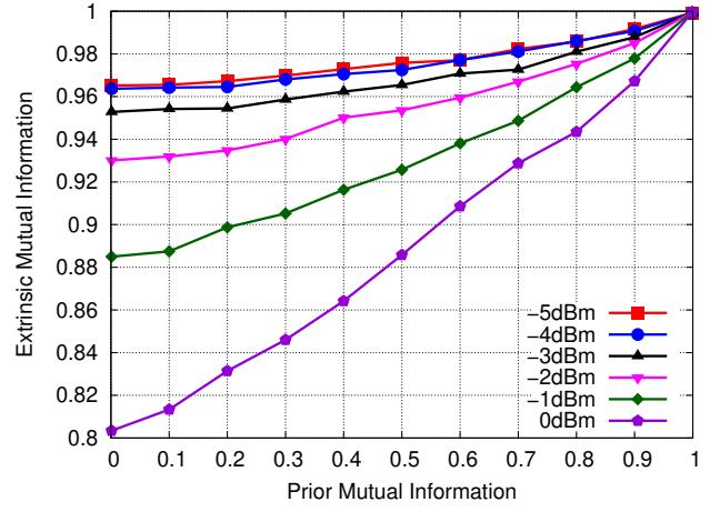
Fig. 4: EXIT chart of DNN-TEQ for DP-16QAM in 16-span DM links.
