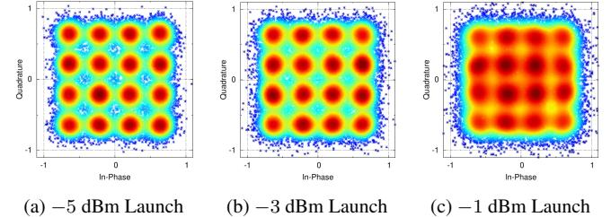
Fig. 2: Residual nonlinear distortion of DP-16QAM constellation after LE for 16-span NZDSF DM links.
