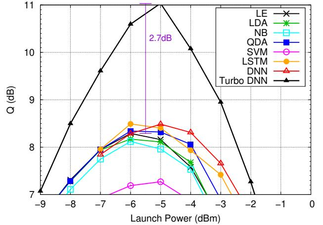
Fig. 6: Single-iteration DNN-TEQ for DP-4QAM 50-span NZDSF (DVB-S2 LDPC code of rate 9/10).
