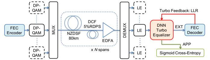
Fig. 1: Coherent optical communications with DNN-TEQ.
