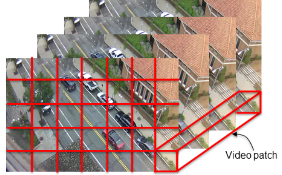
Figure 2: Illustration of a grid of regions partitioning a video frame and a video patch encompassing 4 frames. This figure show non-overlapping regions, but in our experiments we use overlapping regions.
