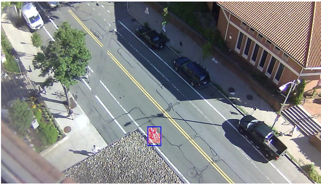
Figure 15: Detection result for flow-based method showing correctly detected biker outside of the bike lane.
