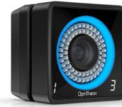
Fig. 2. A camera from the Optitrack motion-capture system used for verifying our control and estimation algorithms.
