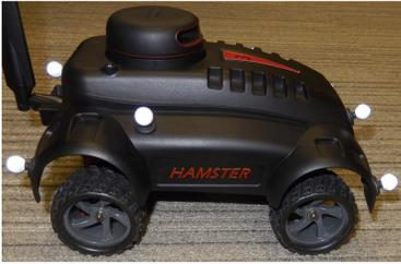
Fig. 1. The Ackermann-steered Hamster mobile robot used in the experiments. The markers (five visible in the figure) are used to track the robot via an Optitrack motion-capture system (Fig. 2).
