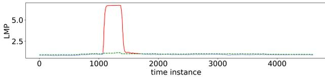
Fig. 4: The LMP values of a faulty testing item and the thresholds determined by baseline LMPs; the green dashed line indicates thresholds, the blue dotted line indicates normal windows in the testing item, and the red solid line indicates faulty windows in the testing item.
