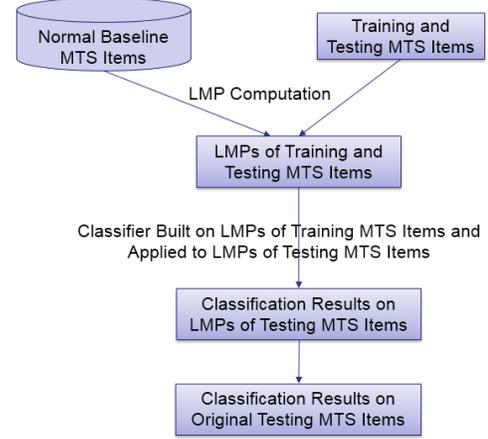
Fig. 2: The structure of the LMP-based fault classifier.
