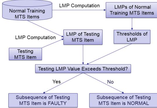
Fig. 1: The structure of the LMP-based fault detector.
