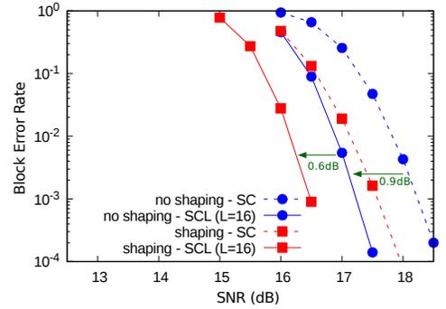
Fig. 4: BICM shaping at medium block length (2.0 bits/dimension, block length: 1024 dimensions).
