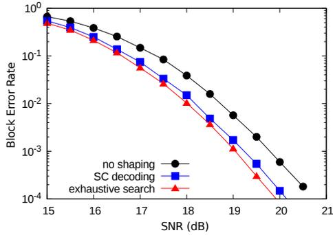
Fig. 3: The effect of decoding schemes used for shaping (2.0 bits/dimension, block length: 64 dimensions).
