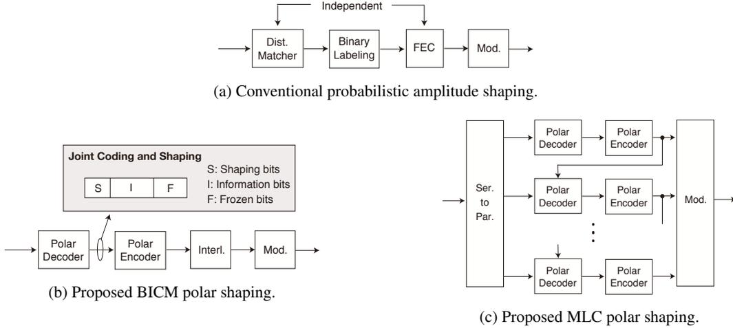
Fig. 1: Encoders of conventional reverse-concatenation shaping schemes based on distribution matcher vs. proposed polar-coded BICM/MLC shaping schemes for joint channel coding and probabilistic shaping.
