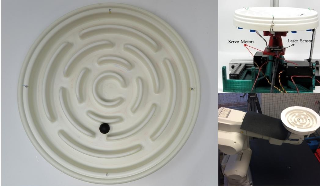
Figure 1: Circular Maze Environment (CME) with a single marble—a toy bought on Amazon. The goal is to maneuver the marble(s) from the outermost ring through a series of gates into the center area. **Right** Experimental platform used for model-based learning, and **Bottom-Right** experimental platform used for transfer learning.
