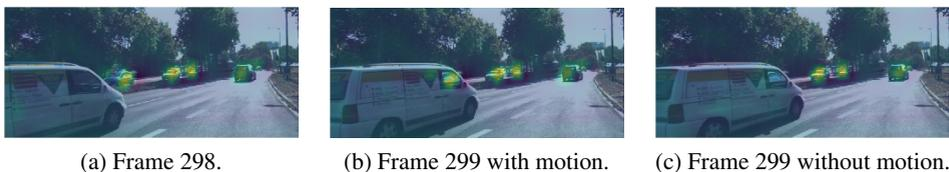
Figure 3: Visualization of the feature map output from the recurrent layer in our RMf-SSD overlaid on input frames. The frames are from video 51 of the KITTI benchmark. The yellow highlights show that when motion information is present in the data (in the form of previous frames) the network responds to cars even if they are heavily occluded in the final frame. Without motion information, the occluded car is missed.
