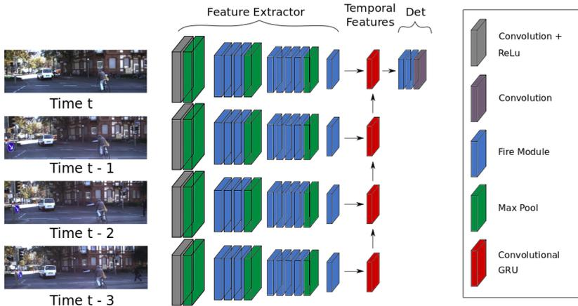
Figure 1: Recurrent Multi-frame Single Shot Detector (Mf-SSD) Meta-Architecture. The depicted RMf-SSD is based on the SqueezeDet+ architecture [34]. RMf-SSDs extend modern, single shot object detection frameworks to the video domain by merging information from sequential images with a convolutional recurrent fusion layer. The *fire module* refers to a specific combination of layers described in the original SqueezeNet paper [17].
