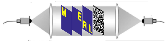
Fig. 1. THz compressed scanning setup for multi-layer imaging of non-overlapping contents.
