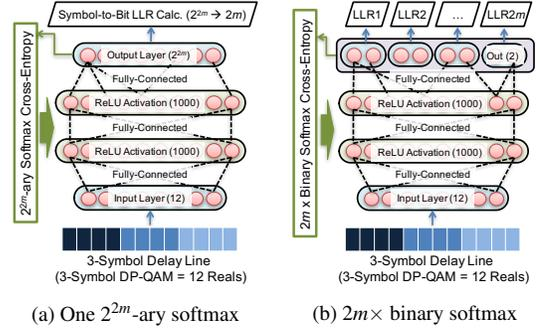
Fig. 2: Single-/multi-label DNN for DP- $2^m$ QAM.
