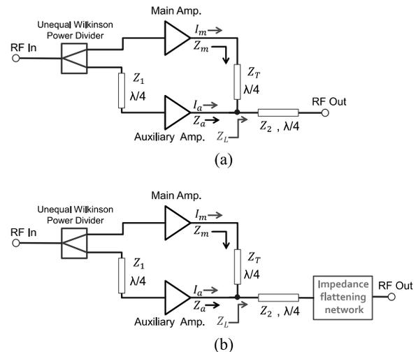
Fig. 1: Block diagram of (a) conventional Doherty power amplifier, (b) proposed wideband Doherty power amplifier with impedance flattening network.
