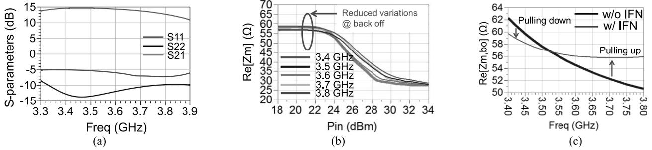
Fig. 4: (a) S-parameter simulation results, (b) real part of  $Z_m$  both at back-off and peak input power, (c) frequency response of real part of  $Z_m$  at back-off with and without impedance flattening network across 3.4-3.8 GHz.
