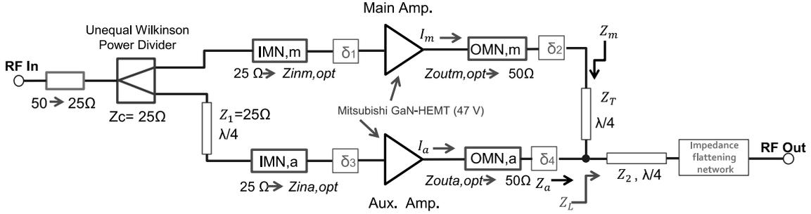
Fig. 3: Complete block diagram of the proposed wideband Doherty power amplifier with impedance flattening network.
