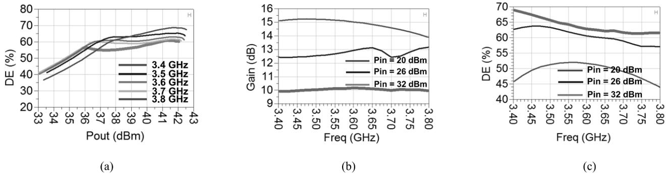
Fig. 5: Large-signal simulation results of proposed wideband Doherty PA (a) output power versus drain efficiency (DE), (b) gain response at 3.4-3.8 GHz, (c) drain efficiency across 3.4-3.8 GHz for various conditions of input power.
