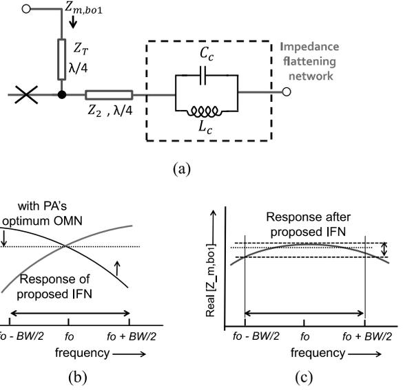
Fig. 2: Block diagram of (a) proposed impedance flattening network (IFN), (b) frequency responses of PA's optimum output matching network in typical condition and proposed IFN alone, (c) resultant frequency response after incorporating the IFN in load modulation network.
