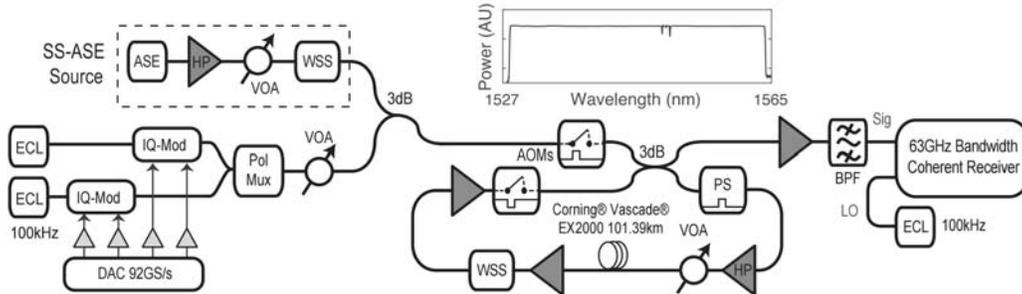
Fig. 1. Experimental setup used in this work. Inset: spectrum for spectrally shaped ASE.
