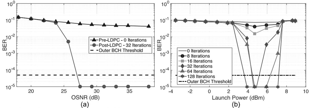
Fig. 2. Experimental results: (a) BER averaged over both subchannels in back-to-back configuration before and after LDPC decoding. (b) BER performance after transmission over 400 km of Vascade EX2000 fiber with full C-band ASE loading. Note that measurements exhibiting no bit errors after LDPC decoding over  $3 \times 10^6$  bits per measurement are rounded up to a BER of  $10^{-5}$ .
