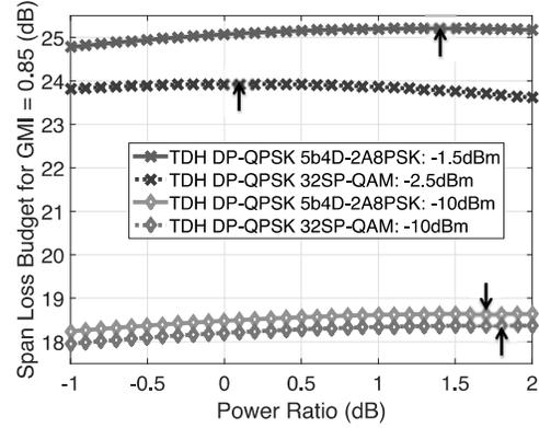
Fig. 5: Span loss budget for the 2A8PSK-based and the conventional TDH at 4.5 bits/symbol, as a function of power ratio, at the nonlinear and linear regions. The arrows indicate the optimum power ratio
