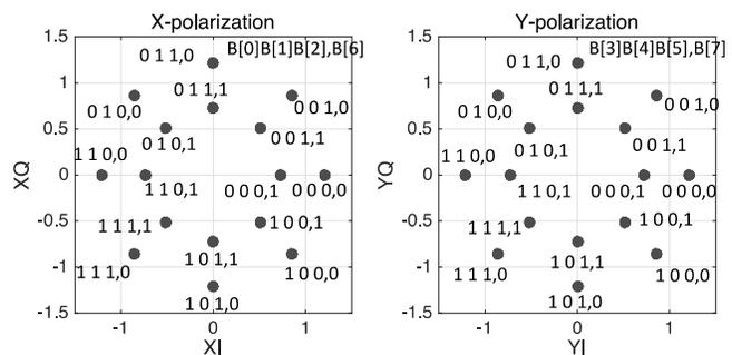
Fig. 1: Constellation and bit-to-symbol mapping of 2A8PSK [10].
