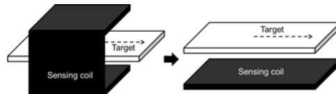
Fig. 1. Left: U-shaped slot sensor. Right: planar sensor.
