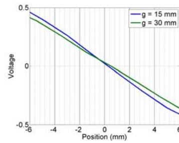
Fig. 6. Experiment measurement result of differential voltage as function of position at different gap sizes.
