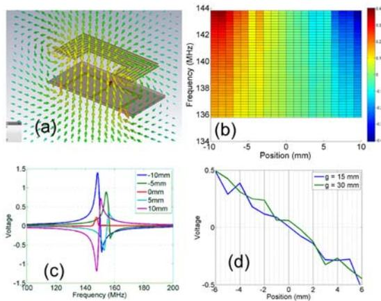
Fig. 4. Simulated results: (a) Field distribution at resonance; (b) Differential voltage mapping as function of target position and excitation frequency; (c) Differential voltage at different positions as function of frequency; (d) Differential voltage as function of position at fixed frequency.
