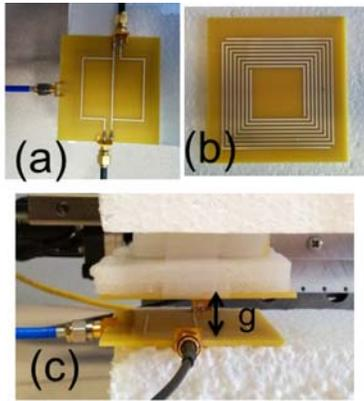
Fig. 5. Fabricated sensing and target coils, and the measurement setup.
