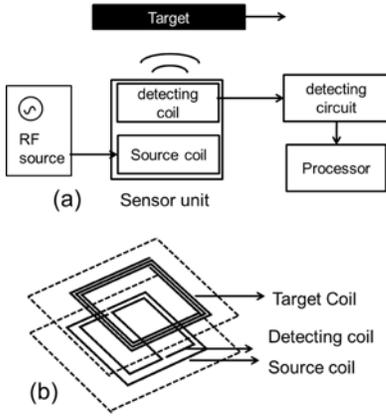
Fig. 2. (a) Block diagram of the proposed sensing system. (b) Example design of sensor structures.
