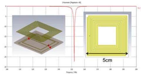
Fig. 3. Simulated reflection to the excitation port around the resonant frequency of the target coil. The structures are shown in the inset.
