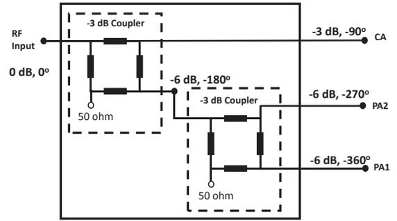
Fig. 3. Schematic of the multi-way splitter of the proposed three-way SPA.
