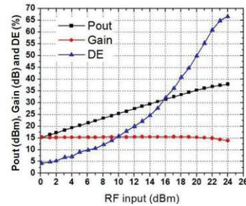
Fig. 5. Measured Pout, Gain, and DE of the carrier amplifier of the three-way SPAs ( $V_{DS} = 20V$ ,  $V_{GS} = -2.8V$ ,  $f = 2.5$  GHz, CW stimulus).
