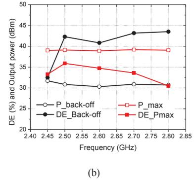
Fig. 8. Measured three-way SPA performance of (a) 2.7 GHz with CW and (b) frequency response under CW signal at peak and 9dB backoff output power.
