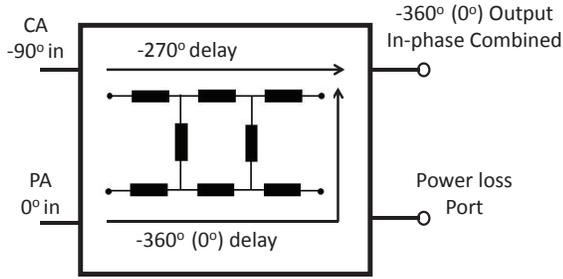
Fig. 2. Schematic of the output coupler of the proposed two-way SPA.
