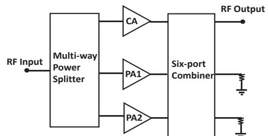
Fig. 1. Schematics of the proposed three-way SPAs.
