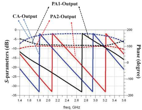
Fig. 6. Measured S-parameter magnitude and phase of the fabricated six-port combiner (7:1.5:1.5) of the three-way SPA.
