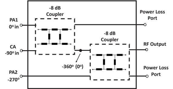
Fig. 4. Schematic of the six-port combiner of the proposed three-way SPA.
