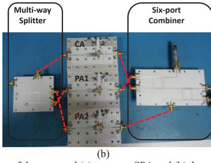
Fig. 7. Top views of the proposed (a) two-way SPA and (b) three-way SPA.
