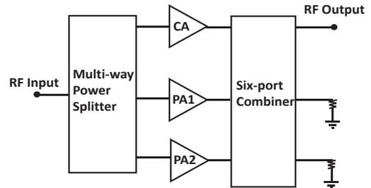
Fig. 1. Schematics of the proposed three-way SPAs.
