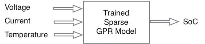
Fig. 1: SoC estimation using sparse GPR.
