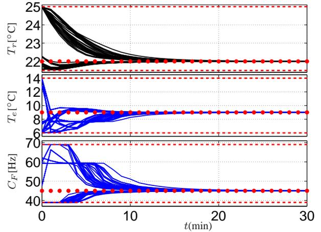
Fig. 3. IAMPC control of air conditioning system. Time trajectories (solid) constraints (dash), setpoint (dot).
