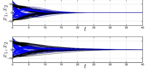
Fig. 2. Simulations with fast ( $c = 1/2$ , upper plot) and slow ( $c = 1/20$ , lower plot) parameter estimator,  $[x]_1$  blue,  $[x]_2$  black.
