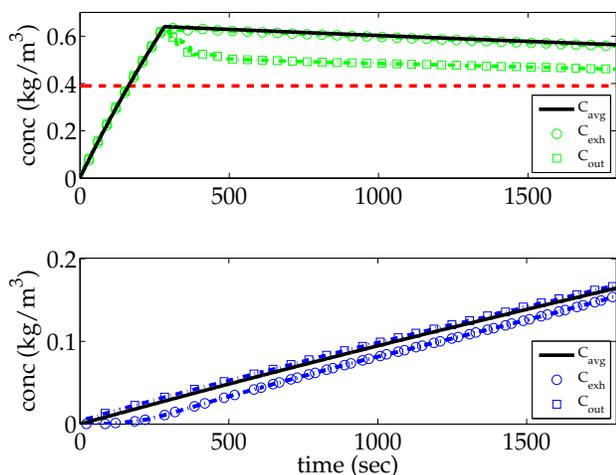
Figure 3:  $\bar{C}$  compared to the local concentrations  $C_{exh}$  and  $C_{out}$  for the high-rate leak (upper plot) and low-rate leak (lower plot).
