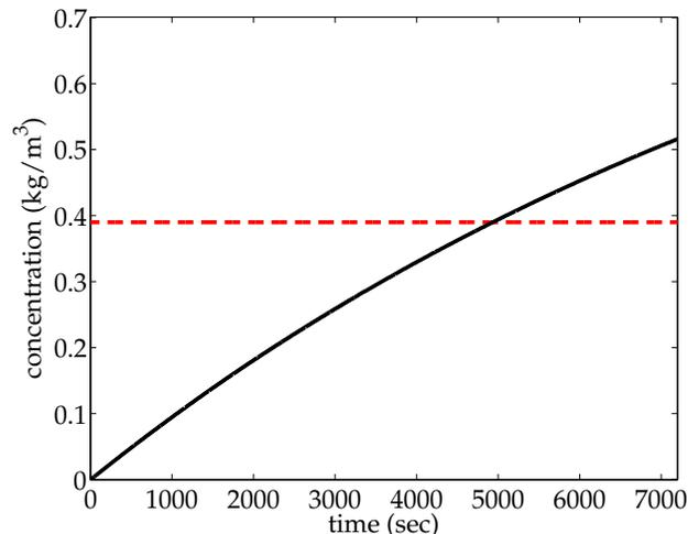
Figure 2:  $\bar{C}$  during a low-rate leak, with  $Q_{exh} = 5$  cfm and  $h_{out} = 0.25$  in, over 7200 seconds. The RCL is denoted by the dashed line.
