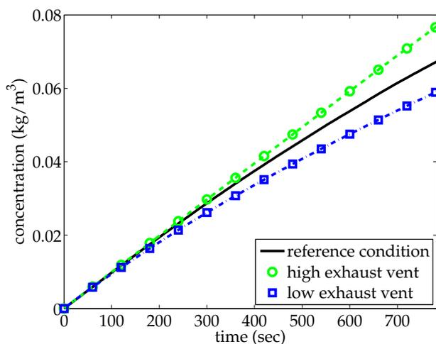
Figure 9:  $\bar{C}$  for different locations of exhaust vent and refrigerant injection.
