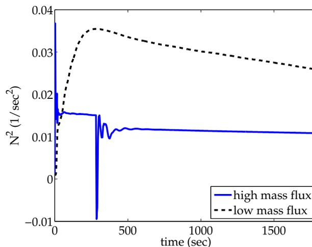
Figure 4: Buoyancy frequency indicates significant stratification.
