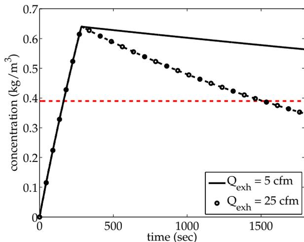
Figure 7:  $\bar{C}$  over 1800 seconds during a high-rate leak for cases where  $Q_{exh}$  varies between 5 cfm and 25 cfm, with  $h_{out} = 0.25$  in. The RCL is denoted by the dashed line.
