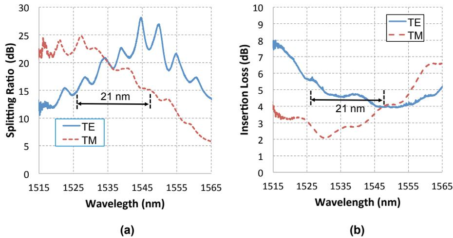
Fig. 2. (a) PBS splitting ratio (SR) and (b) insertion loss (Loss) as a function of the wavelength.
