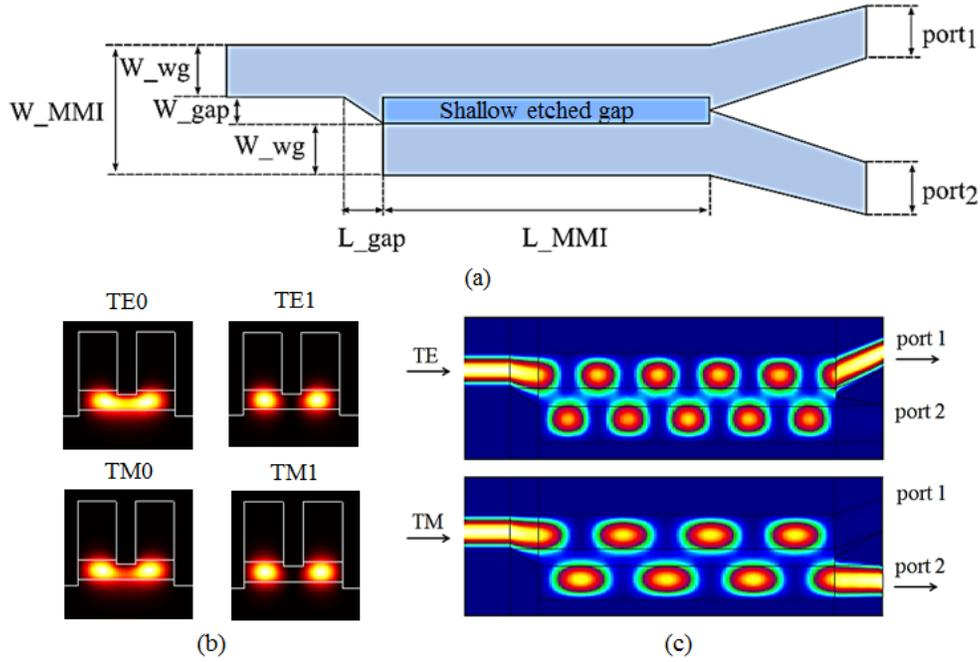
Fig. 1. (a) PBS device scheme. (b) Cross-section view of the MMI TE and TM modes. (c) TE and TM field propagation in the PBS device.
