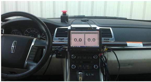
Fig. 7. Lincoln MKS dashboard: the display screen and the GPS receiver installed for in-vehicle testing.
