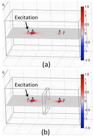
Figure 1: Field intensity in a wireless power system, before and after the introduction of a metamaterial slab. Note that the receive coil on the right is excited much more effectively with the addition of the metamaterial
