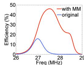
Figure 4: Transfer efficiency versus frequency for metamaterial slab
