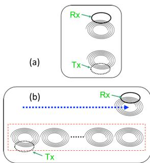
Figure 5: Planar resonator array (schematic view)
