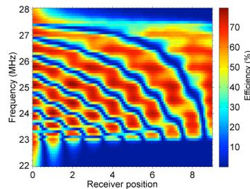
Figure 6: Predicted efficiency of resonant transfer array
