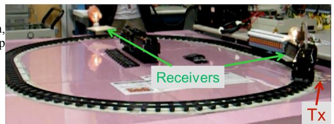
into relatively high voltage (50 – 200 volt) DC, and a switching power supply converted that voltage down to 5VDC to operate the traction motor. A telemetry system uplinked the operating voltages continuously during operation. This system is shown in figure 7. The system operated as predicted, with nulls and peaks as expected; the positions of the nulls were dependent on the RF drive frequency (26.5 to 27.5 MHz).
