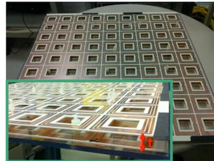
Figure 2: Metamaterial slab
