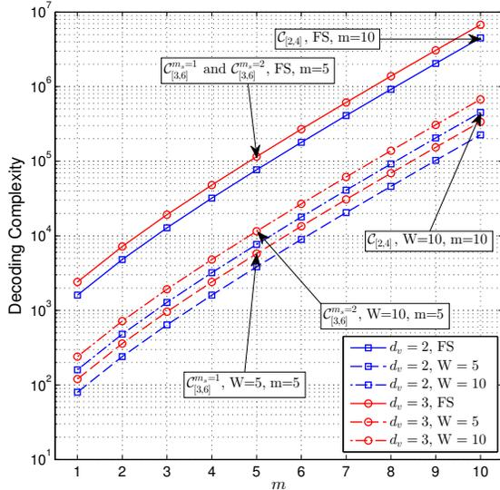
Fig. 5. The order of decoding complexity  $\mathcal{O}(W \cdot c \cdot d_v (q + qm))$  when an LDPC block code and an SC-LDPC code have the same decoding latency and thus have the same decoding complexity.
