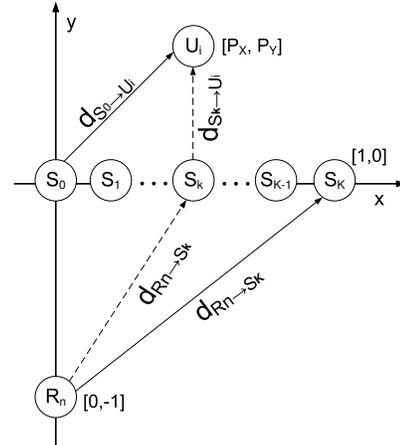
Fig. 2. Linear topology of a multihop cognitive relay network.
