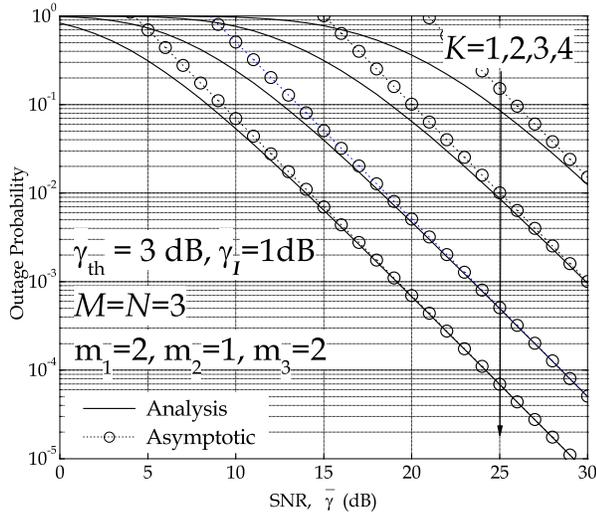
Fig. 5. Outage probability of the cognitive multihop relay network: Effect of the fading severity parameters.
