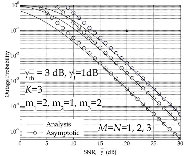
Fig. 4. Outage probability of the cognitive multihop relay network: Effect of the fading severity parameters.
