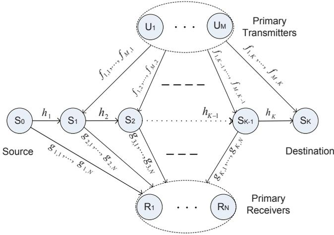
Fig. 1. System model of a cognitive multihop relay network with multiple primary transmitters and receivers.
