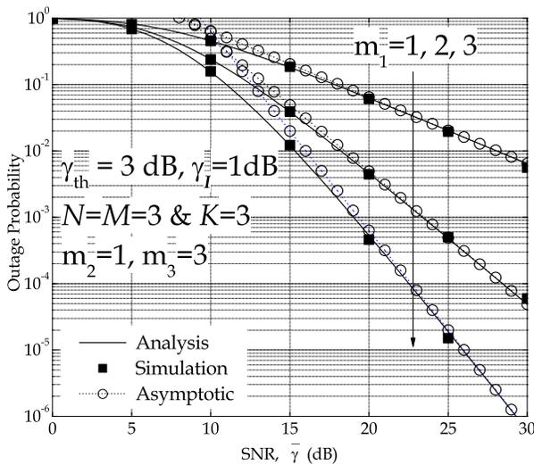
Fig. 3. Outage probability of the cognitive multihop relay network: Effect of the fading severity parameters.
