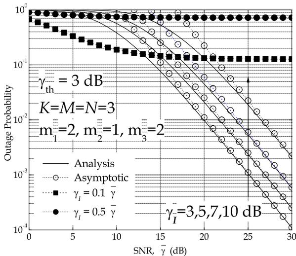
Fig. 6. Outage probability of the cognitive multihop relay network: Effect of the fading severity parameters.
