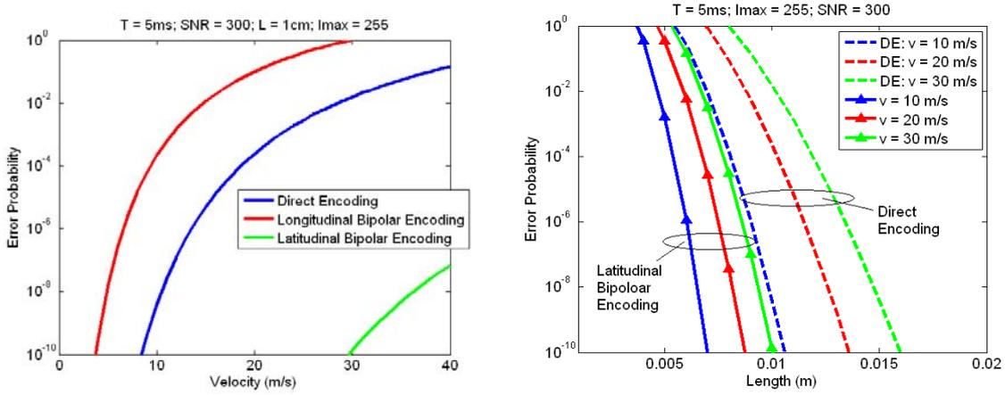
Figure 8 Performance of Latitudinal Bipolar Encoding
