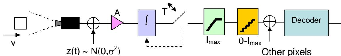
**Figure 5 Model of Image Receiver**
