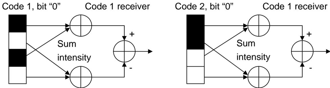
**Figure 4 Differential Decoder**
