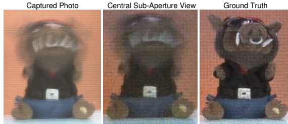
Figure 12: Objects moving faster than the temporal sampling rate results in motion blur in the recovered frames, similar to a video camera.
