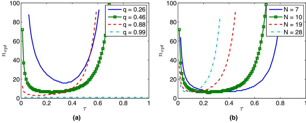
**Fig. 3:** The optimum number of time slots  $n = n_{opt}$  as a function of broadcast probability  $\tau$ , local detection probability  $q$  and network size  $N$  with  $\gamma = 0.95$  confidence threshold: (a) shows  $n_{opt}$  for  $N = 10$  over  $0 \leq \tau \leq 1$  as  $q$  varies; (b) shows  $n_{opt}$  for  $q = 0.46$  over  $0 \leq \tau \leq 1$  as  $N$  takes different values. The case where  $N = 10$  and  $q = 0.46$  is presented in both figures as a reference.
