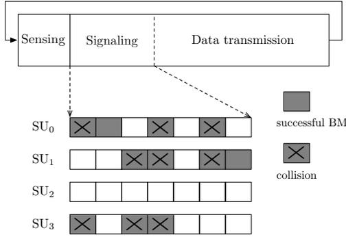
**Fig. 1:** The three phase cognitive cycle and the underlying signaling protocol.
