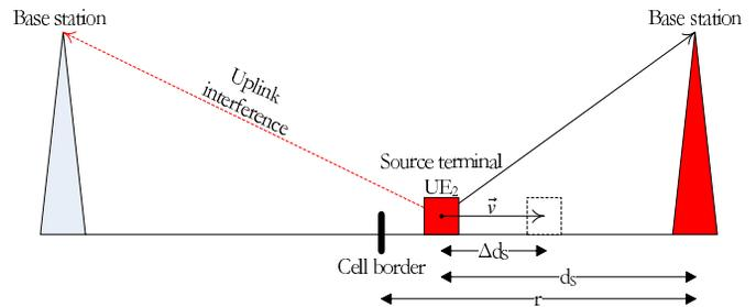
Fig. 1. Illustration of an interference scenario for an uplink transmission in an FDD system during a unit observation interval  $\Delta t$ . In this scenario the source is denoted by  $UE_2$ , whereas the victim is the base station on left hand side.
