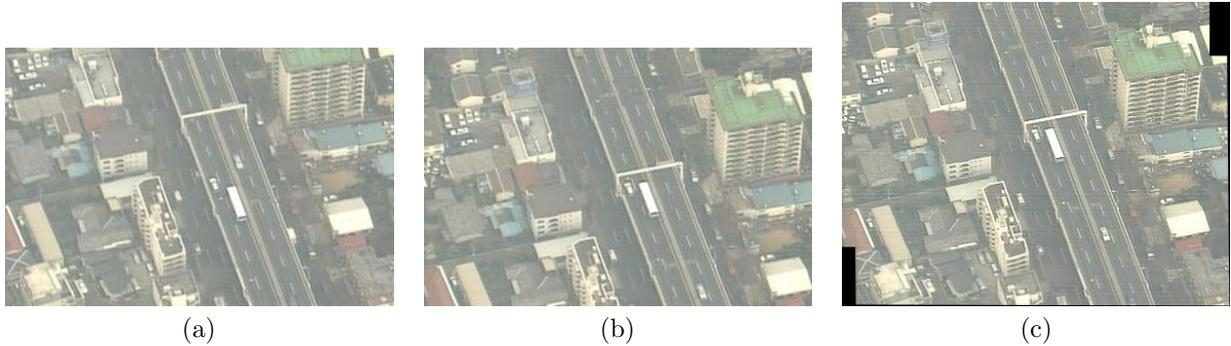
**Figure 1.** Registration result of two aerial images using the affine motion model. In the two images, there are several moving vehicles in the image. The registration result shows the robustness of our proposed algorithm to outliers. (a)(b) are the image pair to be registered. (c) is the registered image.
