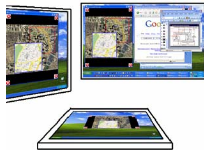
Figure 3. MVI-II: Reflective. The 3 surfaces are running 3 instances of a layered map viewer application. Interactions on any surface are reflected across all surfaces. The lenses on all surfaces display the same layered geospatial data.
